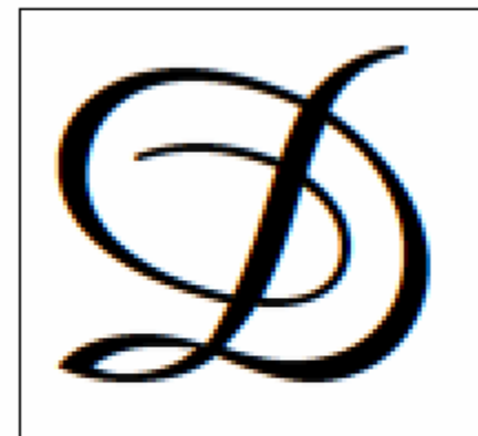
ClearType with Ydirection Antialiasing smooths out the jaggies on shallow curves and other ydirection features
